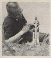
Two V-1 engines are used as strap-ons to provide a big boost to a Valkyrie-2 rocket. All these engines fire at lift-off; at burn-out the two strap-on engines drop off while the central "Sustainer" rocket continues to spectacular altitudes.
